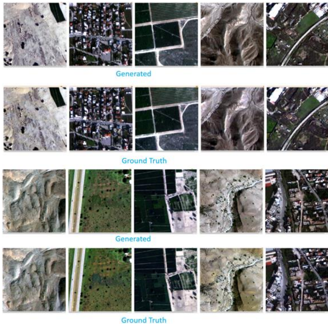
Fig. 2 Images generated by Generator from our proposed approach with PAN, NIR, Red, Green bands as inputs, can be visualized to a variety of test samples.
