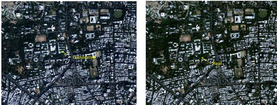
Fig. 3 Blue band generation for part of Ahmedabad scene of Cartosat-3 satellite. Left is Generated blue band replaced RGB image and right is input Ground Truth RGB images.
